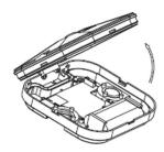
3. AC mains wiring to the luminaire can be done via the M20 flexible soft adaptor to the base or via the snap on cable grommet supplied with the product.
