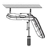
This luminaire is a class II, non-maintained emergency luminaire and only requires mains active and neutral wiring. Close the top cover after mains wiring.
