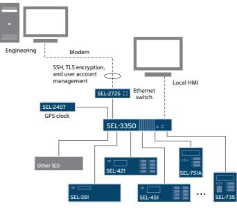
Above: typical topology for a protocol converter or SCADA data concentrator
