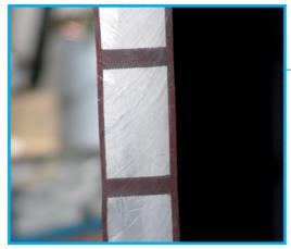
Vacuum casting process allows uniform distance between windings
