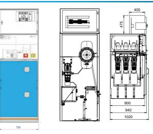
A protection panel with vacuum circuit breaker (ISM type) with a separate hinged door top mounted LV compartment containing a protection relay.
