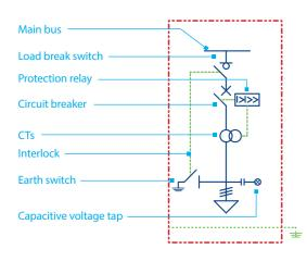
Easily test cables without disconnecting
