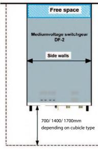
Side plates must be installed running to the wall to create an enclosed free space
