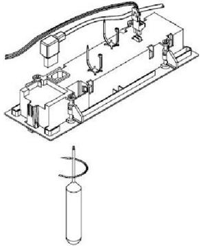
Figure 1: Tight cam lock screw using Philips screwdriver
